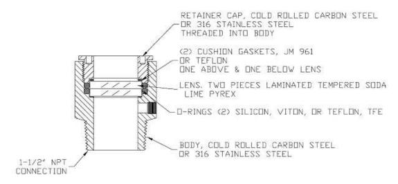
This unit is assembled at the factory and is ready for installation to a vessel. This sight glass should be visually checked for any possible damage during shipping. To install the unit, thread the male NPT end into the vessel and tighten. Tighten the retainer cap into the body with a spanner wrench. This sight glass is now operational.
