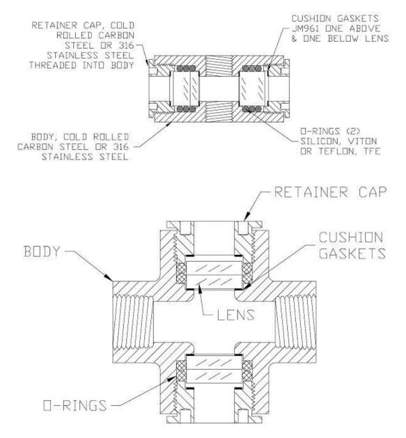
This unit was assembled at the factory and is ready for installation. The sight glass should be visually checked for any possible damage during shipping. To install the unit, thread connecting pipe into the female NPT connection and tighten. Tighten the retainer cap to the body with a spanner wrench. The sight glass is now operational.
