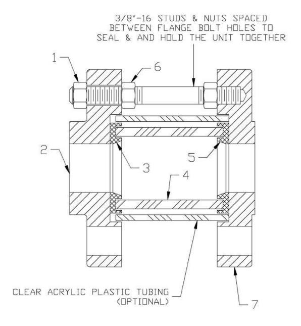
This unit is assembled at the factory and is ready for installation into pipeline. This sight glass should be visually checked for any possible damage during shipping. After the unit has been installed, heated and pressurized, it should be checked for any possible leakage. If leakage occurs, follow steps (h) and (f) until leakage has stopped.
