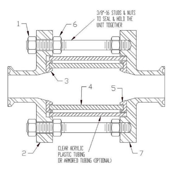
This unit is assembled at the factory and is ready for installation into pipeline. This sight glass should be visually checked for any possible damage during shipping. After the unit has been installed, heated and pressurized, it should be checked for any possible leakage. If leakage occurs, follow step (i) and (j) until leakage has stopped.
