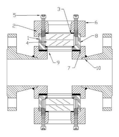
This unit was assembled at the factory and is ready for installation. NOTE: The sight glass should be visually checked for any possible damage during shipping. Alter the unit has been installed; heated and pressurized several times it should be inspected to check for any possible leakage. Ii leakage occurs, follow step (M) until leakage has stopped.
