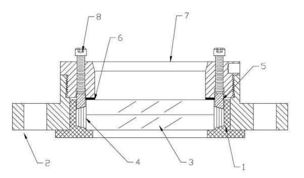
This unit was assembled at the factory and is ready for installation. The packing in this unit was not, and cannot be, fully compressed at the factory because of the units' design. Mount the unit in position, and compress the packing according to Step (I) of these instructions. Follow the steps below when installing new parts.
