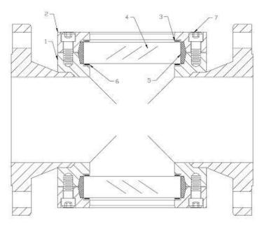
This unit was assembled at the factory and is ready for installation. The sight glass should be visually checked for any possible damage during shipping. After the unit has been installed, heated and pressurized several times, the cap screws holding the retainer cap in place should be checked for tightness.
