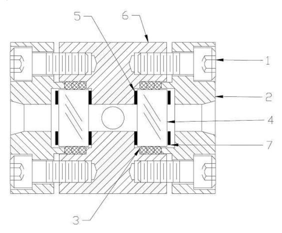
This unit was assembled at the factory and is ready for installation. The sight glass should be visually checked for any possible damage during shipping.
